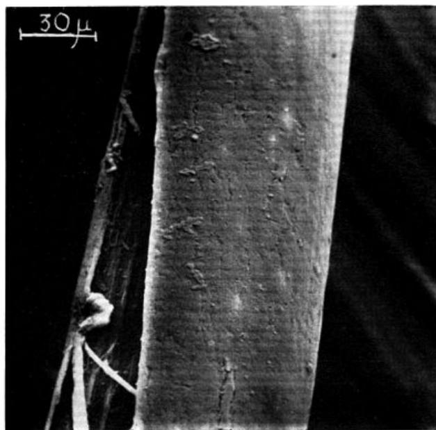
Figure 4. A longitudinal split near the end of a fibre.  $\times 480$ .
