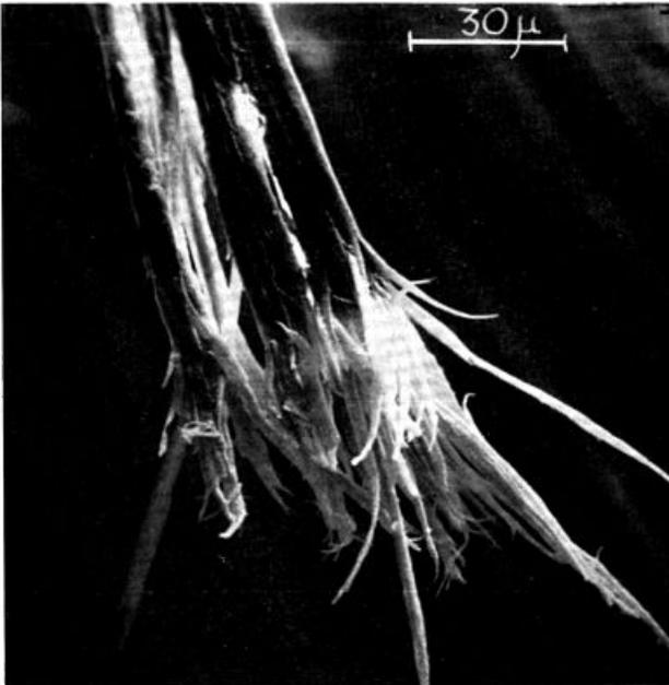
*Figure 6.* A fibrillated end fibre caused by the rupture of a fibrillating region.  $\times 640$ .
