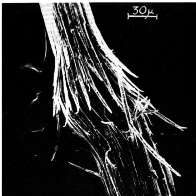
*Figure 8.* Shaft damage in permanently-waved hair. This damage was detected about 10 cm from the end of the fibre.  $\times 400$ .
