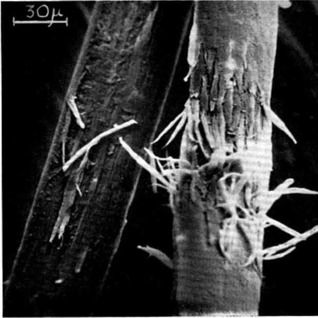
*Figure 5.* A hemicylindrically split fibre segment, fibrillating at cortical cell boundaries.  $\times 480$ .
